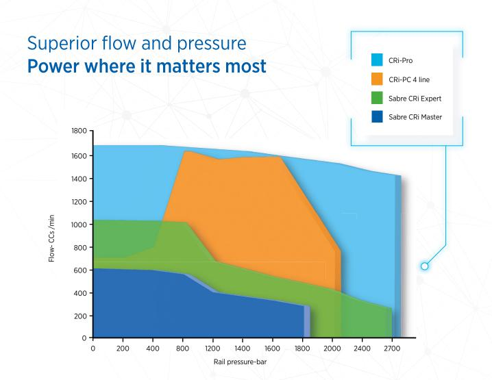
The CRi-Pro hydraulic operating envelope shows the CRi-Pro delivering optimum hydraulic performance at all levels of flow and rail pressure to cater to even the most demanding injectors.
